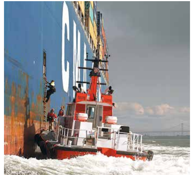
The run boat Golden Gate performs a "change off the Front" pilot exchange. Smooth boat handling in the tricky fluid dynamics alongside deep draft ships is a skill that takes years to master.
