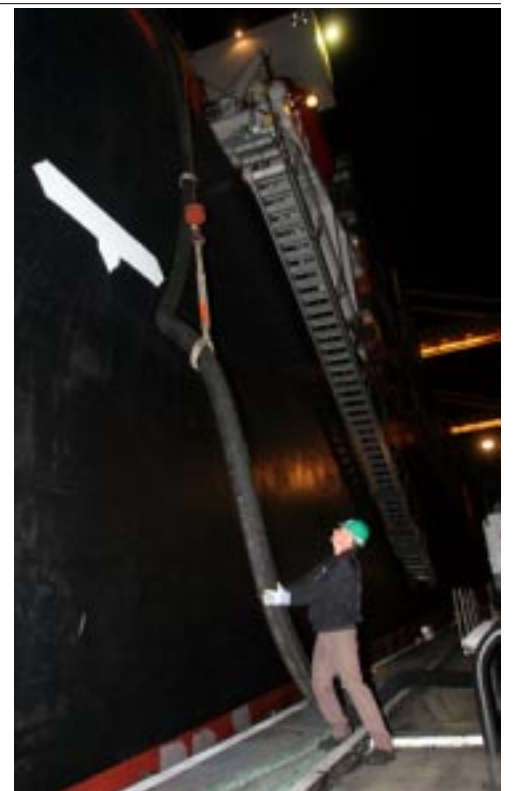
Longtime SUP tankerman Harold Presswood steadies a hose through which oil will be pumped to a cargo ship at the Port of Oakland.
