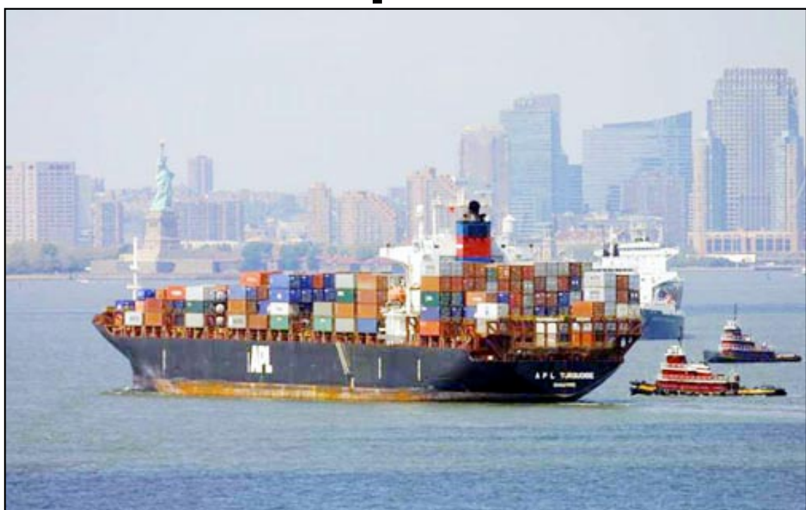
The APL Turquoise pictured entering New York is a 4,468 teu containership built in Japan in 1996. She has a length overall of 964 feet with a beam of 105 feet. Her deadweight tonnage is 59,780 and she is designed to make 24.3 knots.
