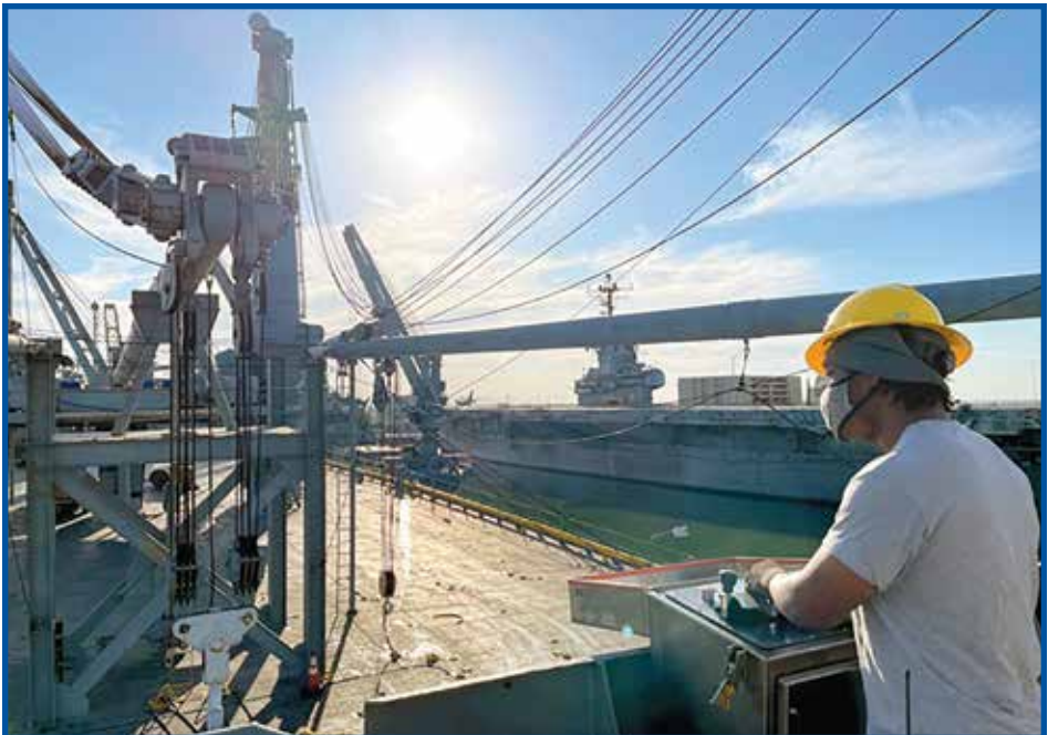
Under the guidance of Bosun Joel Schor, SUP General Vessel Assistant Brandon Hubbard learns the operation of yard and stay gear on Ready Reserve ship Admiral Callaghan in Reduced Operating Status in Alameda California. The museum ship CVN-12 USS Hornet is in the background.
