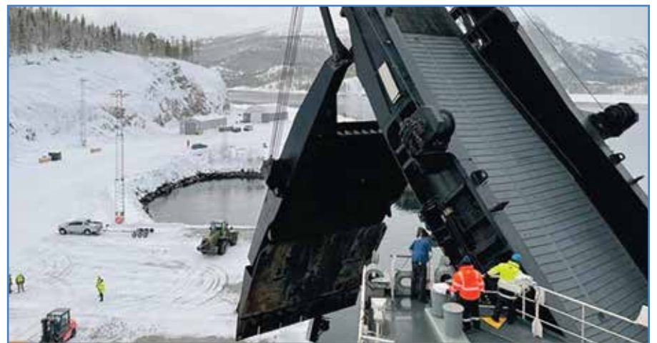
SUP crew deploying the stern ramp alongside berth.
