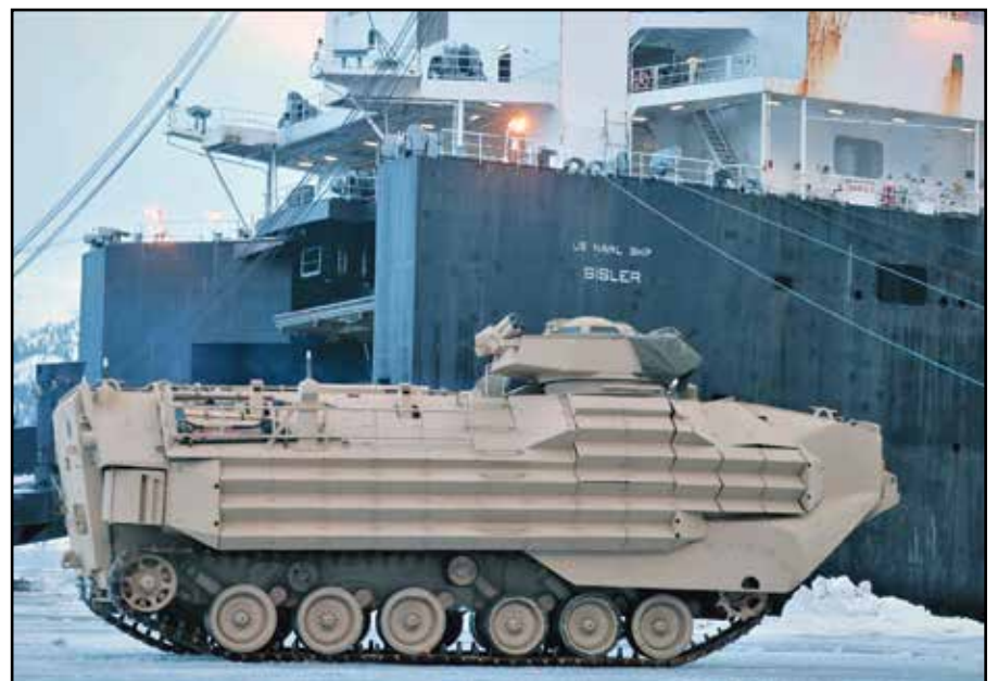
Cargo ashore: the tracked and seaworthy Amphibious Assault Vehicle (or AAVP-7A1 (Personnel)) is offloaded for the exercise. The AAVP, the most common AAV, carries a turret equipped with an M2HB .50 caliber heavy machine gun, and a Mk19 40mm automatic grenade launcher. It has four crew radios as well as the AN/VIC-2 intercom system. It can carry 25 combat equipped Marines in addition to the crew of 3: driver, crew chief/vehicle commander (also the gunner), and rear crewman.
