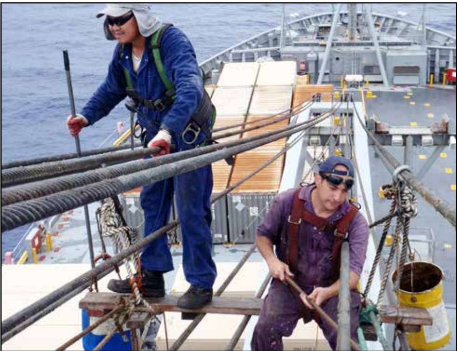
Bosun Cosme Bigno, and AB Andrey Didkovsky slushing the topping lifts on the crane on the USNS Watkins. The Watkins is operated by SUP-contracted Patriot Contract Services for the Military Sealift Command.
