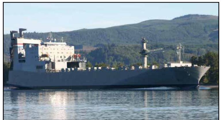
Pictured above is the MV Cape Horn . She and her sister ships Cape Henry and Cape Hudson carry up to 6,766 TEU’s with a 39-ton crane to unload the containers. The Horn has a fixed 63.9-ton capacity vehicle ramp on the starboard/stern quarter which allows Ro/Ro operations to the starboard side or aft only. The vessel has an overall capability of carrying 180,000 square feet of cargo. The ship was built for Norway’s Barber Steamship Company in 1979 and named Barber Tonsberg . She was purchased by the Maritime Administration in 1986, and renamed Cape Horn (T-AKR 5068). The Horn , Henry and Hudson are managed by Matson Navigation Company.
