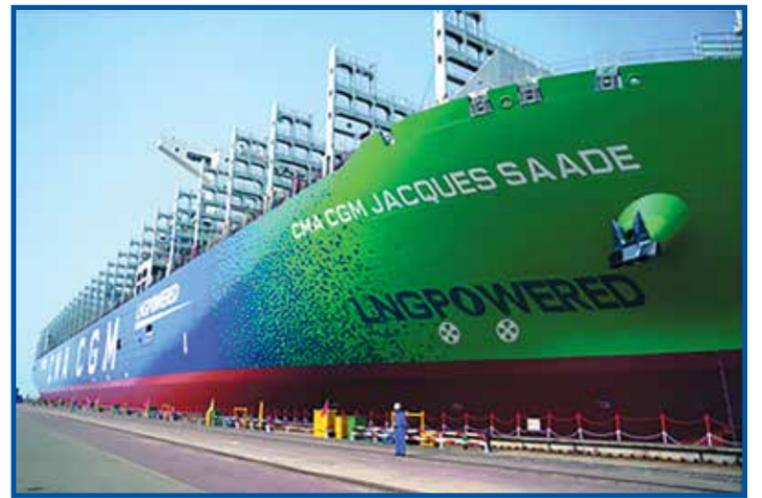
TEU container ships, including the Jacques Saadé class which were the first large LNG-fueled containership ships. CSSC's shipyards built a total of nine of the vessels which each have a capacity of just over 23,000 TEU.
