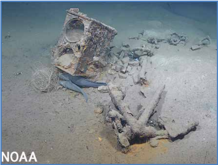
The “tryworks” of the shipwreck Industry , a cast iron stove with kettles used to boil whale blubber into oil.
