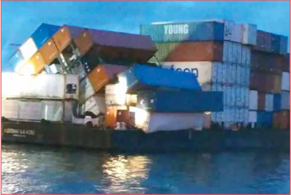
Container collapse on the barge Ho Omaku Hou, part of the inter-island tug service provided by a subsidiary of Foss Maritime Co. Investigation pending.
