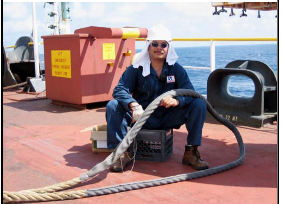
Able Seamen Edgar Paderes onboard the S/R American Progress demonstrates his meticulous seamanship skills by sewing a chafing gear around the eye of a mooring line. SeaRiver vessels typically use expensive Kevlar mooring lines and by applying a protective covering, the line and eye should have a longer service life. Edgar has been a member of the ESU since his employment in 2001 and makes his home in Houston, Texas.
