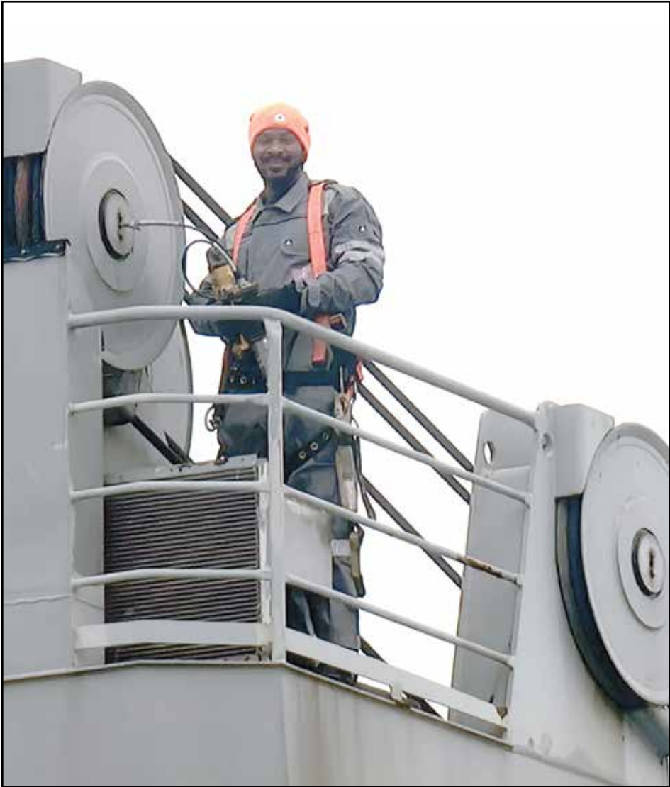
OS Marquese Mitchell greasing the haggling cranes on the USNS George Watson in Baltimore, Maryland.
