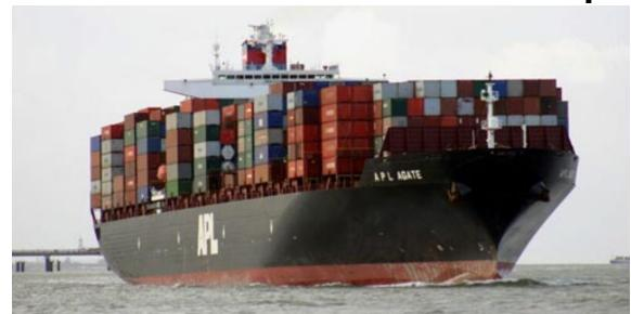
The APL Agate (ex NOL Agate) is a 5,020 teu containership built by Samsung Heavy Industries in 1997 in South Korea. The Agate can make 24.5 knots and is 63,693 deadweight tons.
