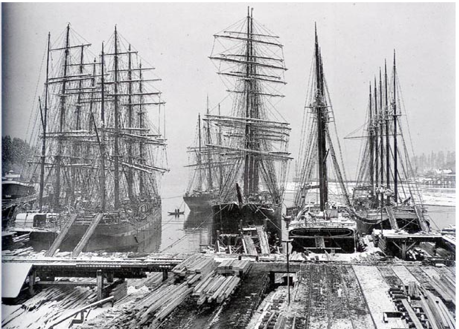
Port Blakely Mill Company dock, Puget Sound, in the winter of 1905. The SUP-crewed vessels from left are: the four-masted barks Englehorn and Bracadale, the barks Albania and Wanderer and the schooners Lyman D. Foster and Crescent. Note the stern ramps to load lumber. Photo by Wilhelm Hester.
